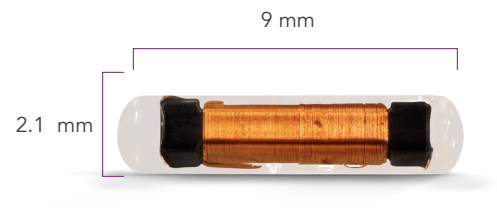
Fig. 2. Image of a microtransponder in which all its components can be seen.
